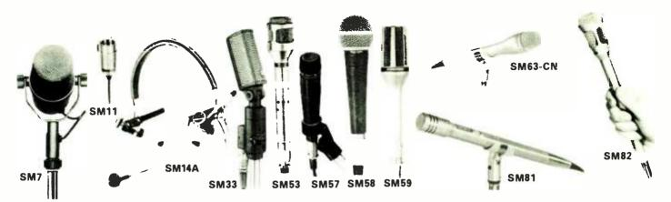
Model SM7: A dynamic microphone with a very smooth, flat, wide-range frequency response; cardioid polar pattern, uniform with frequency and symmetrical about the axis; internal "air suspension" shock isolation; highly effective pop filter; extremely good rejection of electro-magnetic hum due to a built-in hum rejection system; bass rolloff and mid-range emphasis. The Model SM7 was field-designed to be the finest dynamic microphone available for music recording and reproduction.
