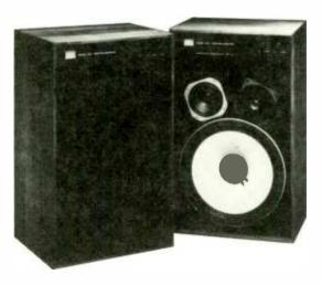
Model 4312 Control Monitor Smooth, powerful, wide-range response within a compact enclosure Components: 300 mm (12 in), long excursion, low frequency loudspeaker 130 mm (5 in) midrange loudspeaker; 36 mm (1.4 in) high frequency direct radiator Mirror-imaged for better stereo imaging 90° dispersion allows vertical or horizontal placement If ordered singly specify left or right \$378.00
